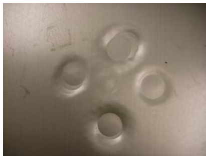
Figure 23: Pipe Impact Test Results
