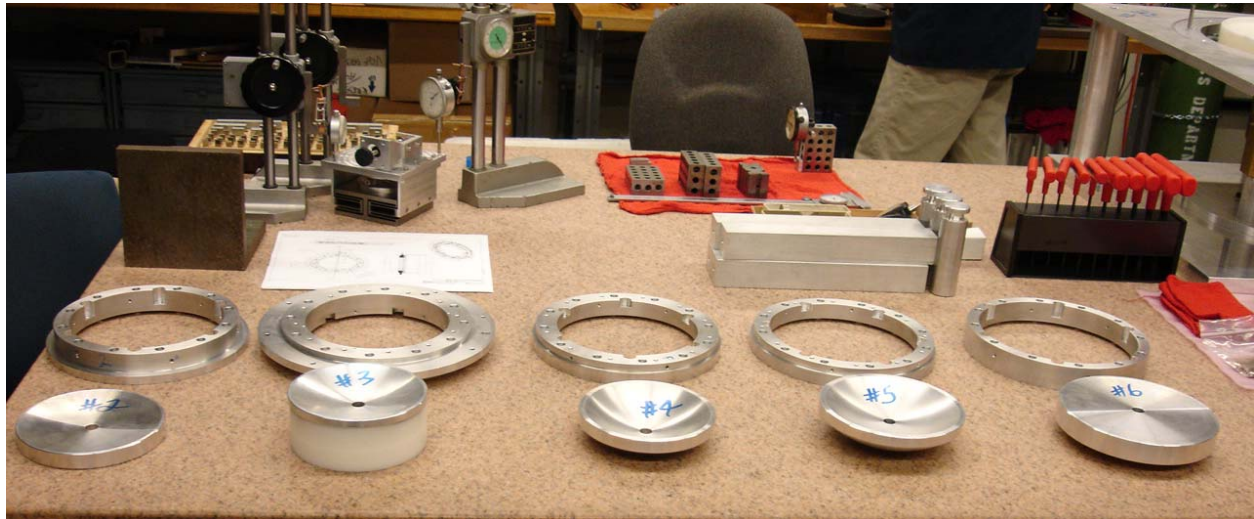
Figure 41: Prototype Collimator Lens Mounts and Dummy Lenses
