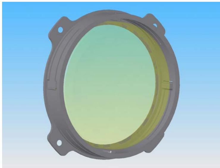
Figure 56: Field Flattener Lens and the Finger-style Lens Support Tabs
